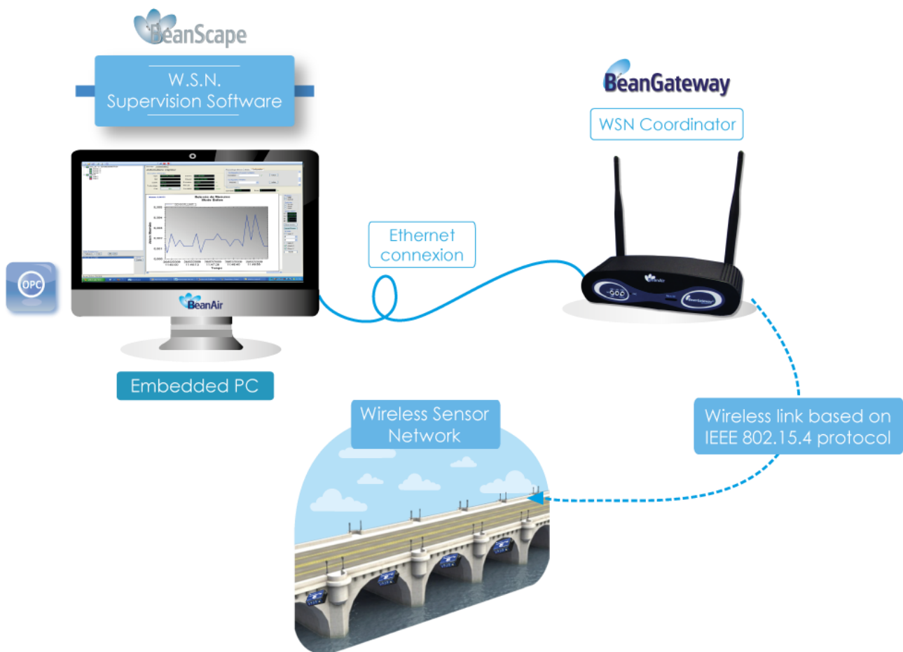
Figure 5: Network Topology with 1 BeanGateway® connected to the BeanScape®
