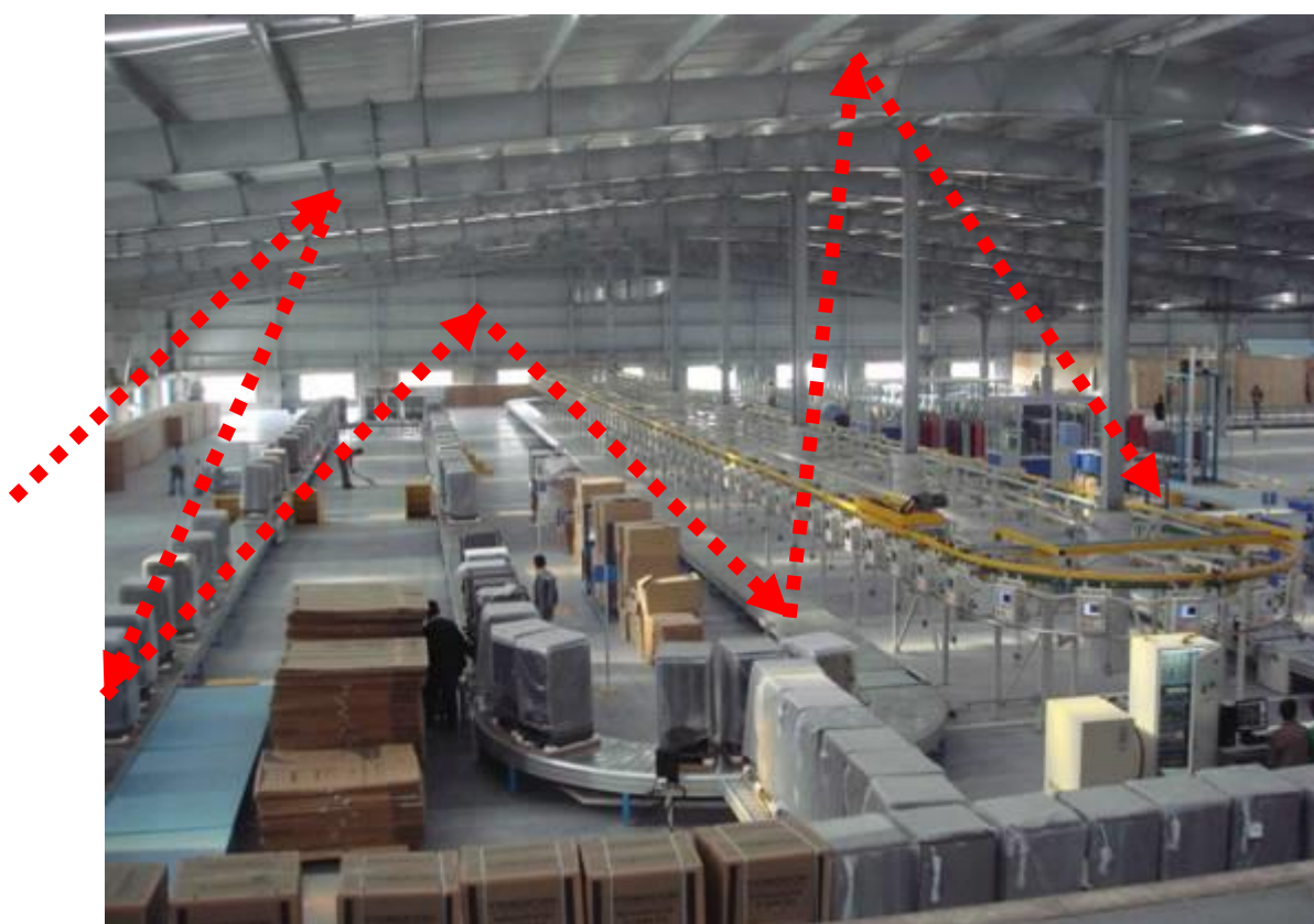
Figure 7: A Simple Multipath Situation in a factory
