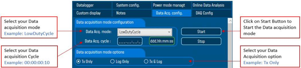
Figure 19 : DAQ Configuration
