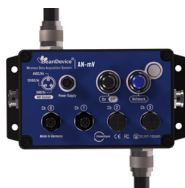
BeanDevice® 2.4GHz AN-V Wireless Analog Data Acquisition System with analog voltage inputs ( \pm 5V ou \pm 10V )
