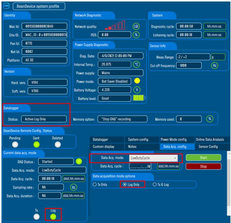
*Figure 10: Configuration of LDCDA mode with Log only option*
