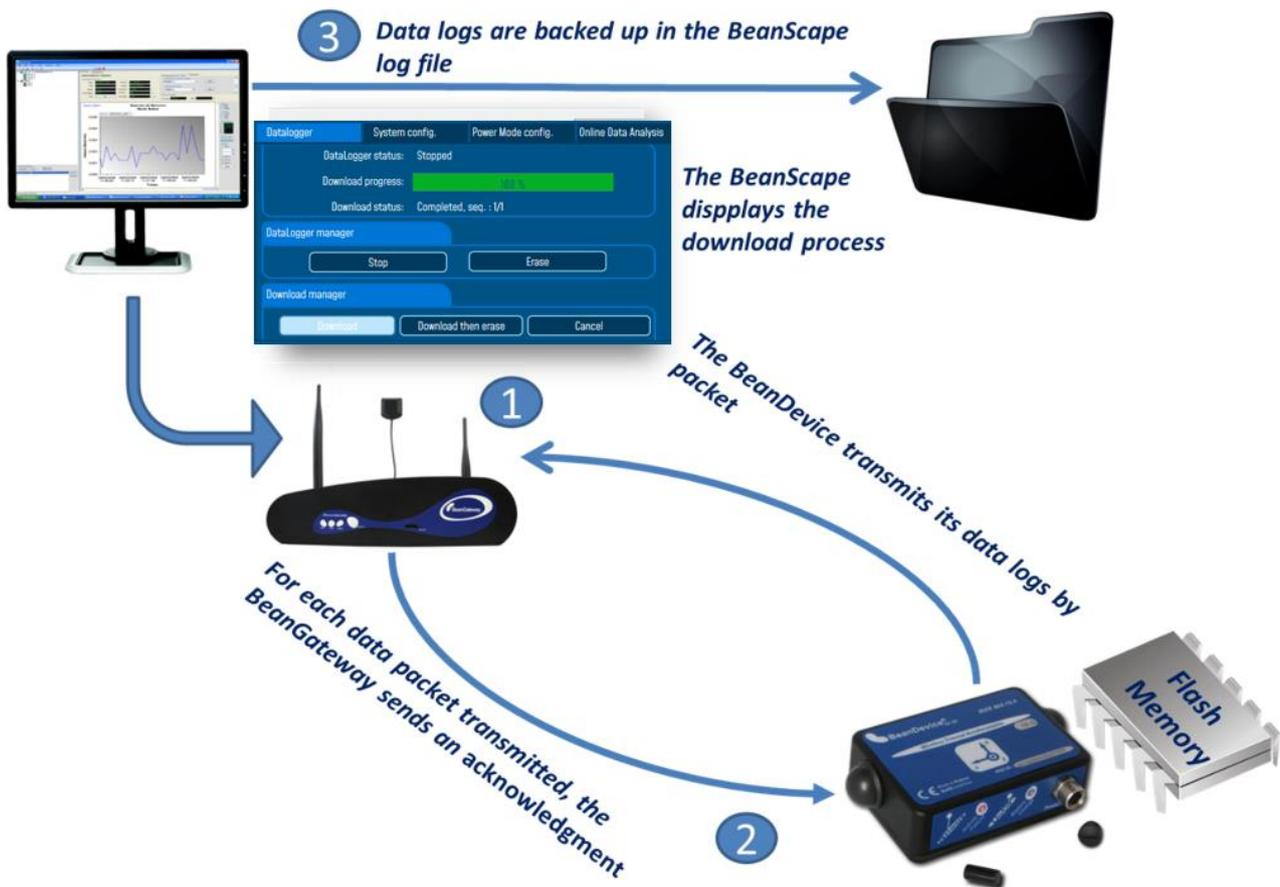
Figure 7: DataLogger download process
