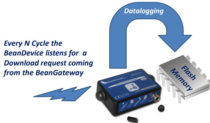
**Figure 4: Data logging without data transmission**
