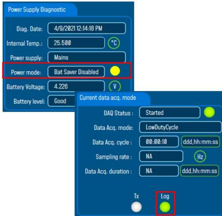
*Figure 12: Log LED when powering on the BeanDevice®*
