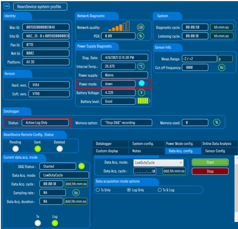
*Figure 11: Power down the BeanDevice® with log only option*
