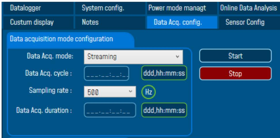
**Figure 106: Right sampling rate for good resonance frequency monitoring**
