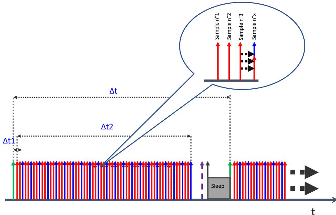
**Figure 5: Streaming mode with “Burst” option timeline**
