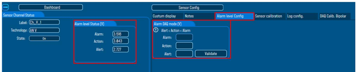
Figure 42: Overview Alarm thresholds (S.E.T mode)
