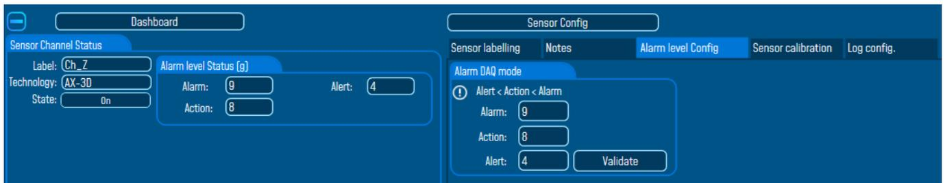
**Figure 40: S.E.T mode Alarm threshold configuration**
