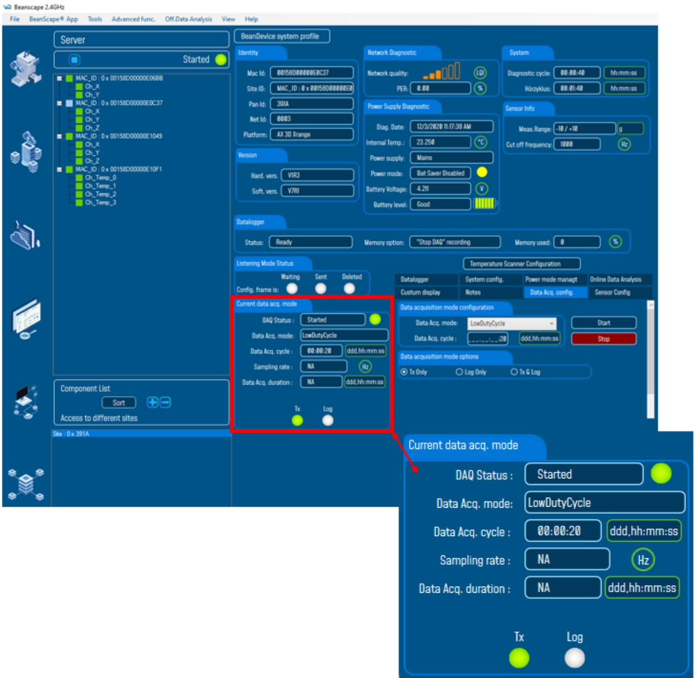
Figure 18: Current data acquisition mode tab
