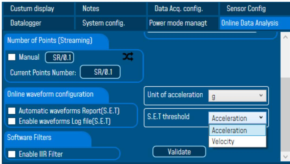
*Figure 93: Setting the type of threshold (S.E.T mode)*
