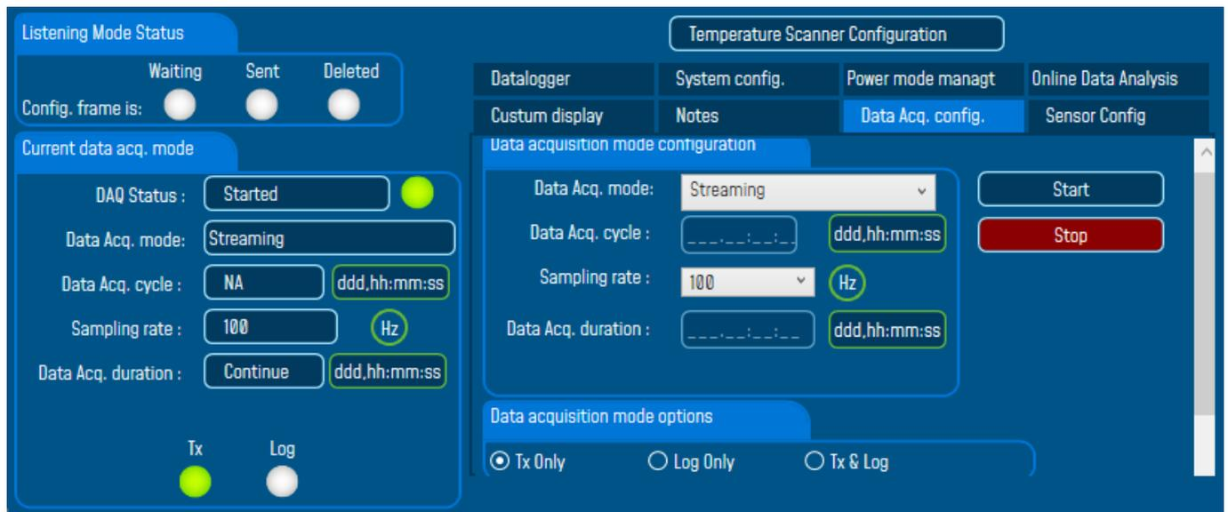
*Figure 104: Wrong sampling rate value for resonance frequency monitoring*
