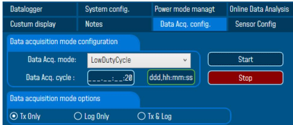
*Figure 19 : Low Duty cycle Data acquisition configuration Tab*
