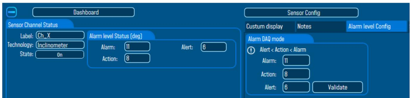
**Figure 35: Alarm thresholds (Survey mode)**
