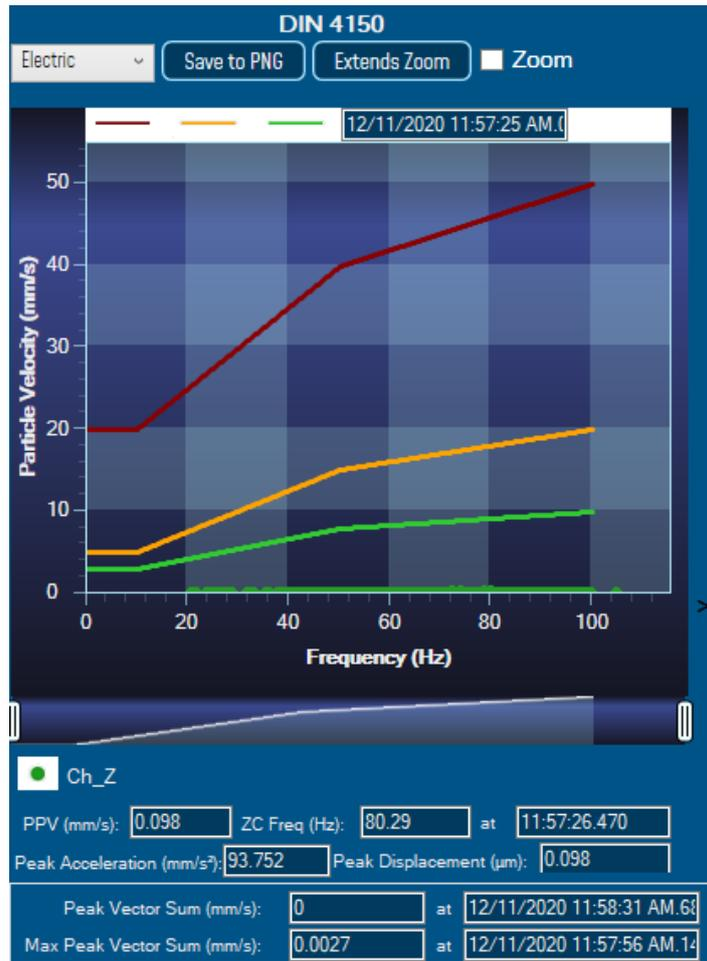
Figure 76: DIN 4150 Real Time Graph, PPV & PVS
