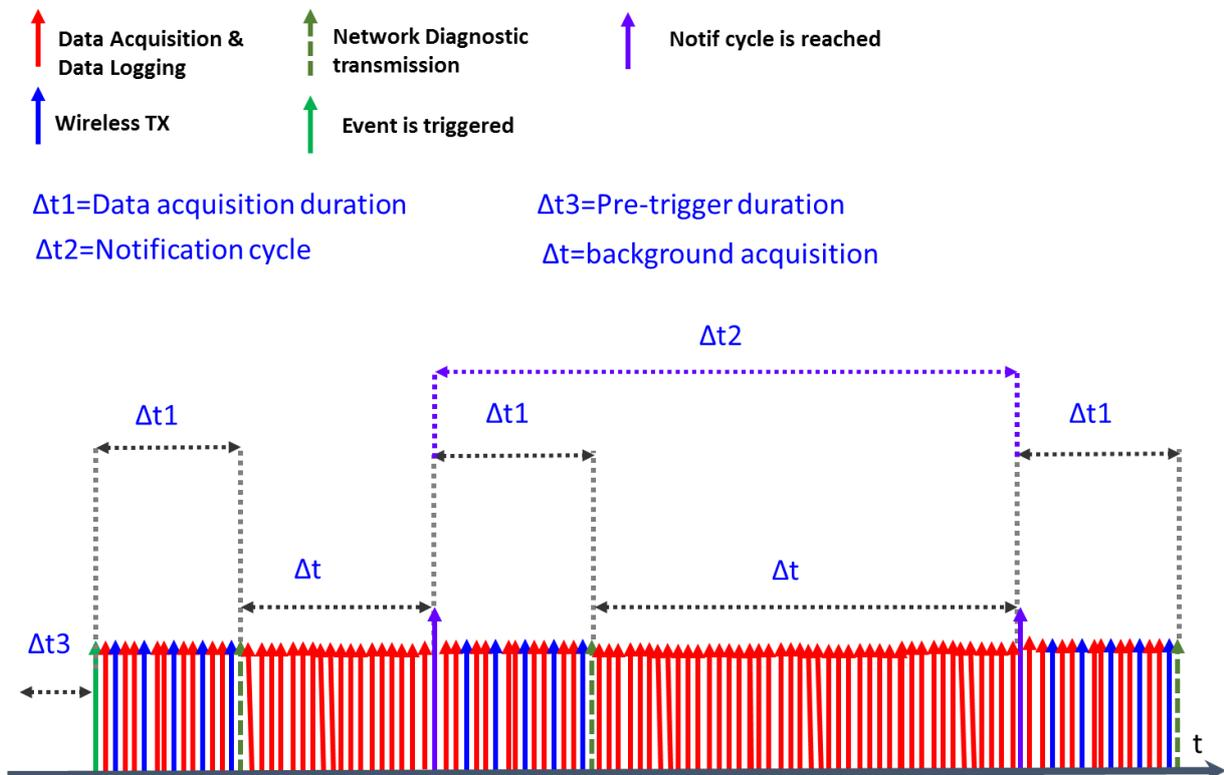
**Figure 6: Streaming with event trigger (S.E.T.) mode timeline**
