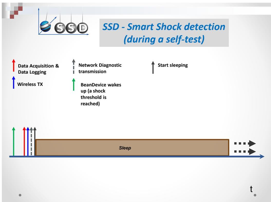
**Figure 8: SSD Mode timeline during a self test**
