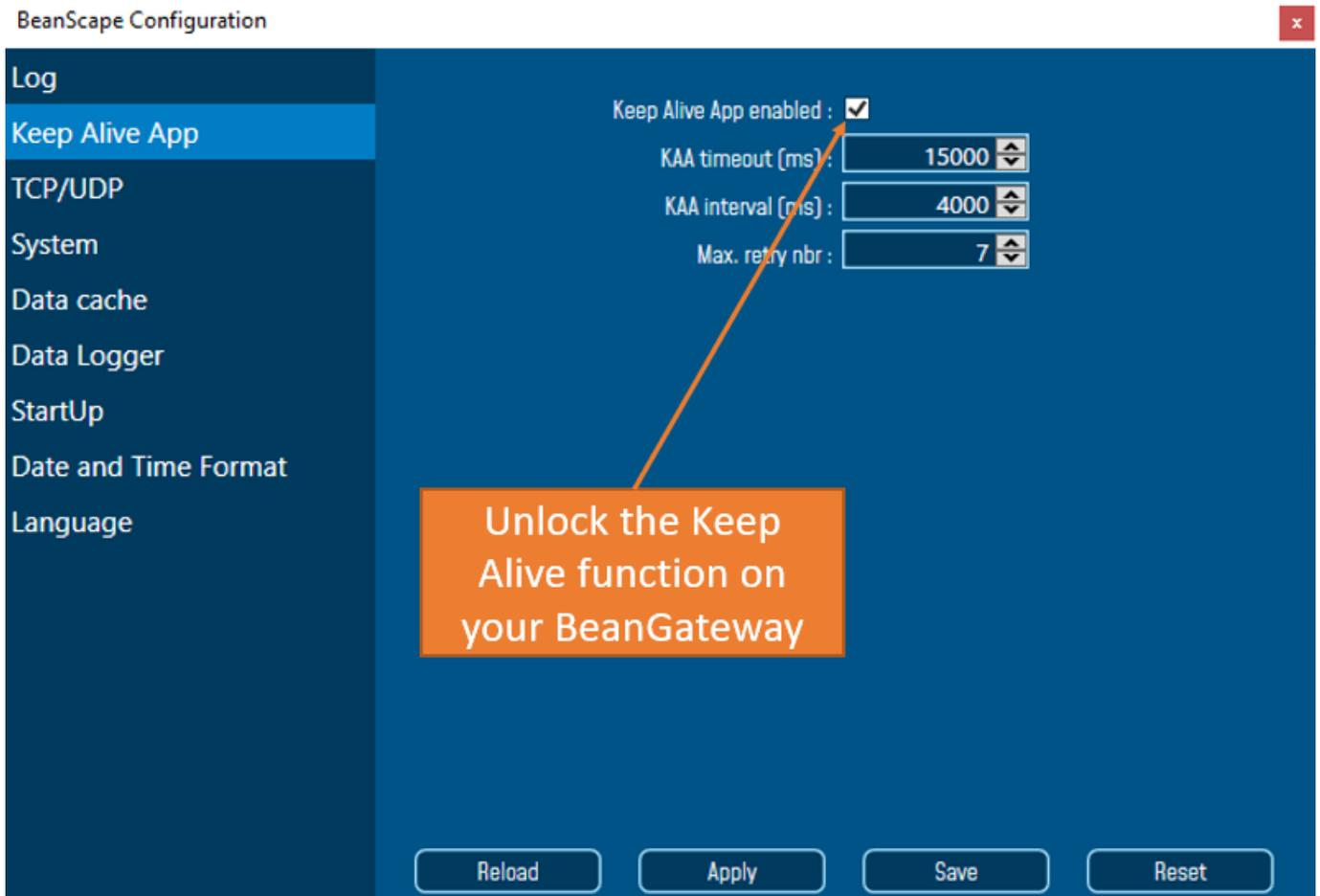
*Figure 111: KeepAlive option on BeanScape configuration window*
