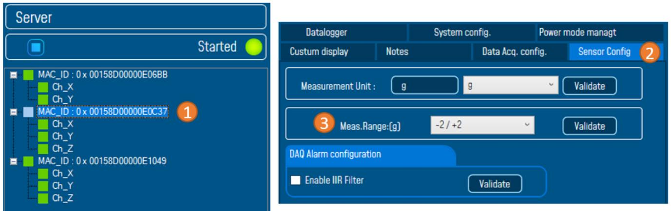
*Figure 89: Sensor measurement range configuration*
