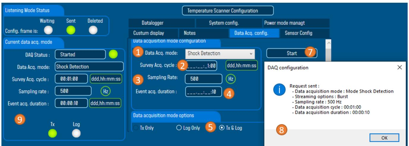
**Figure 91: Overview: Shock Detection mode configuration**
