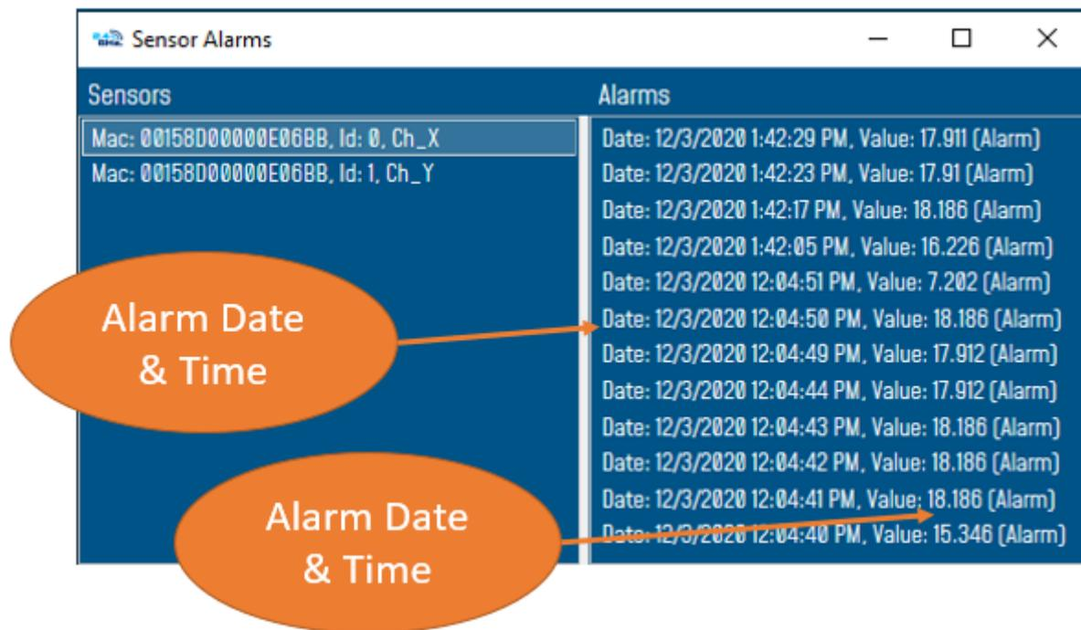
**Figure 34: Exceeded thresholds displayed on Sensors alarms window**
