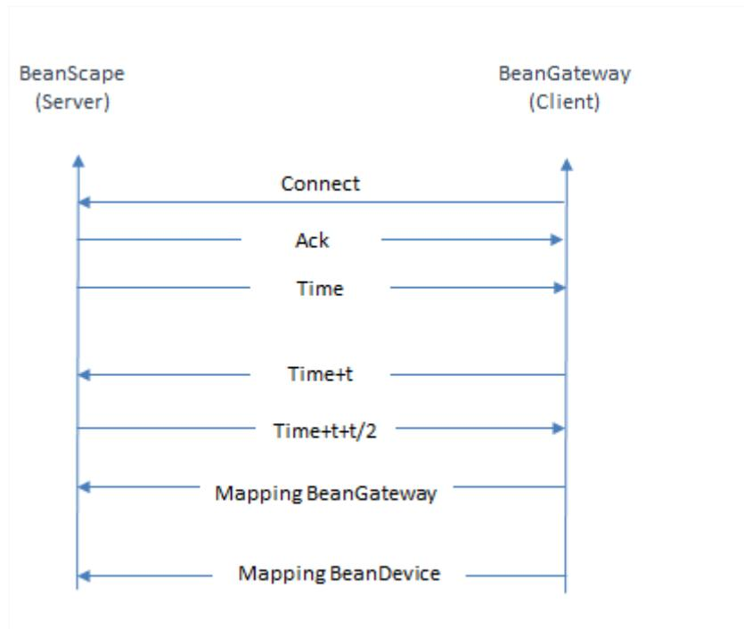
The time synchronization process between the BeanGateway® and the BeanDevice® is described in the following flowchart.
