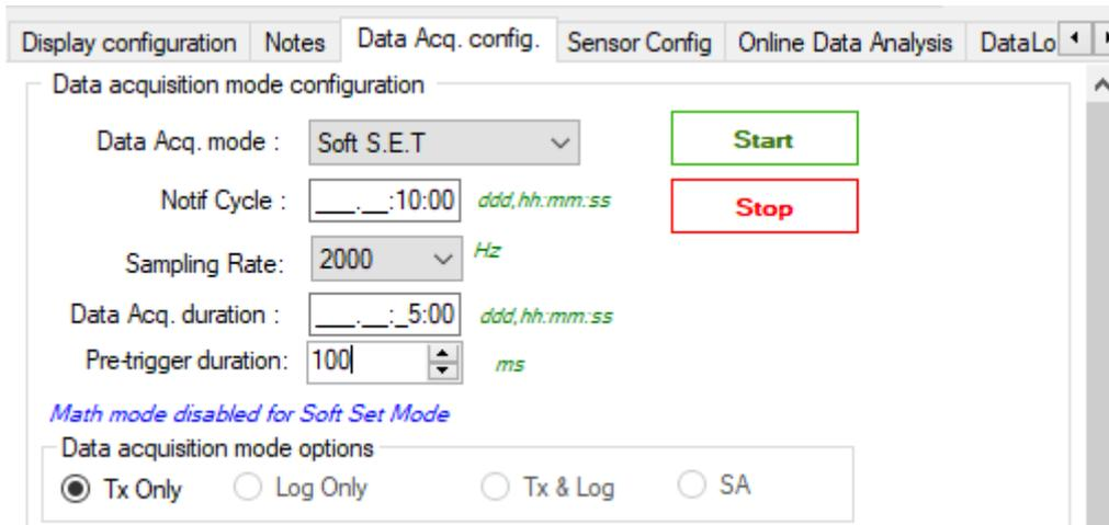
**Figure 22: Soft S.E.T Mode Data acquisition configuration tab**
