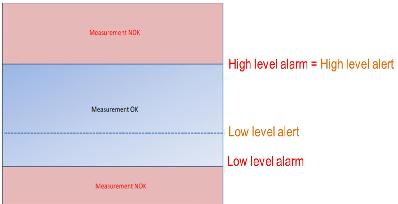
**If (High level alarm > High level alert) & (Low level alert = Low level alarm)**
