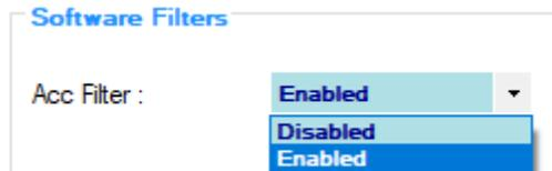
The acceleration filter is used to reduce the noise and makes the signal smooth.
