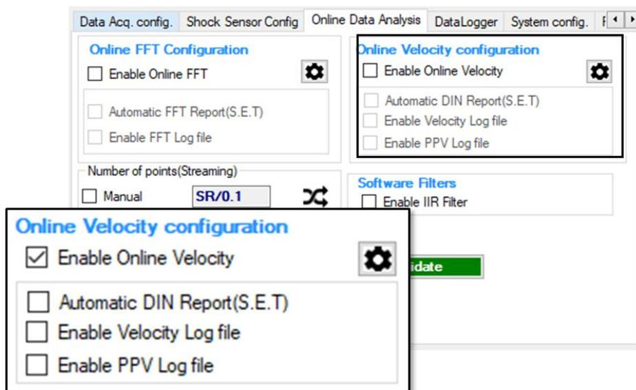
**Figure 73: Online Velocity configuration tab**
