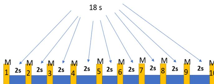
$$\text{Math Notif Cycle} = (\text{Data Acq Cycle} \times \text{Tx\_Ratio} \times \text{Math.NotifRation}) - \text{Data Acq.cycle}$$
