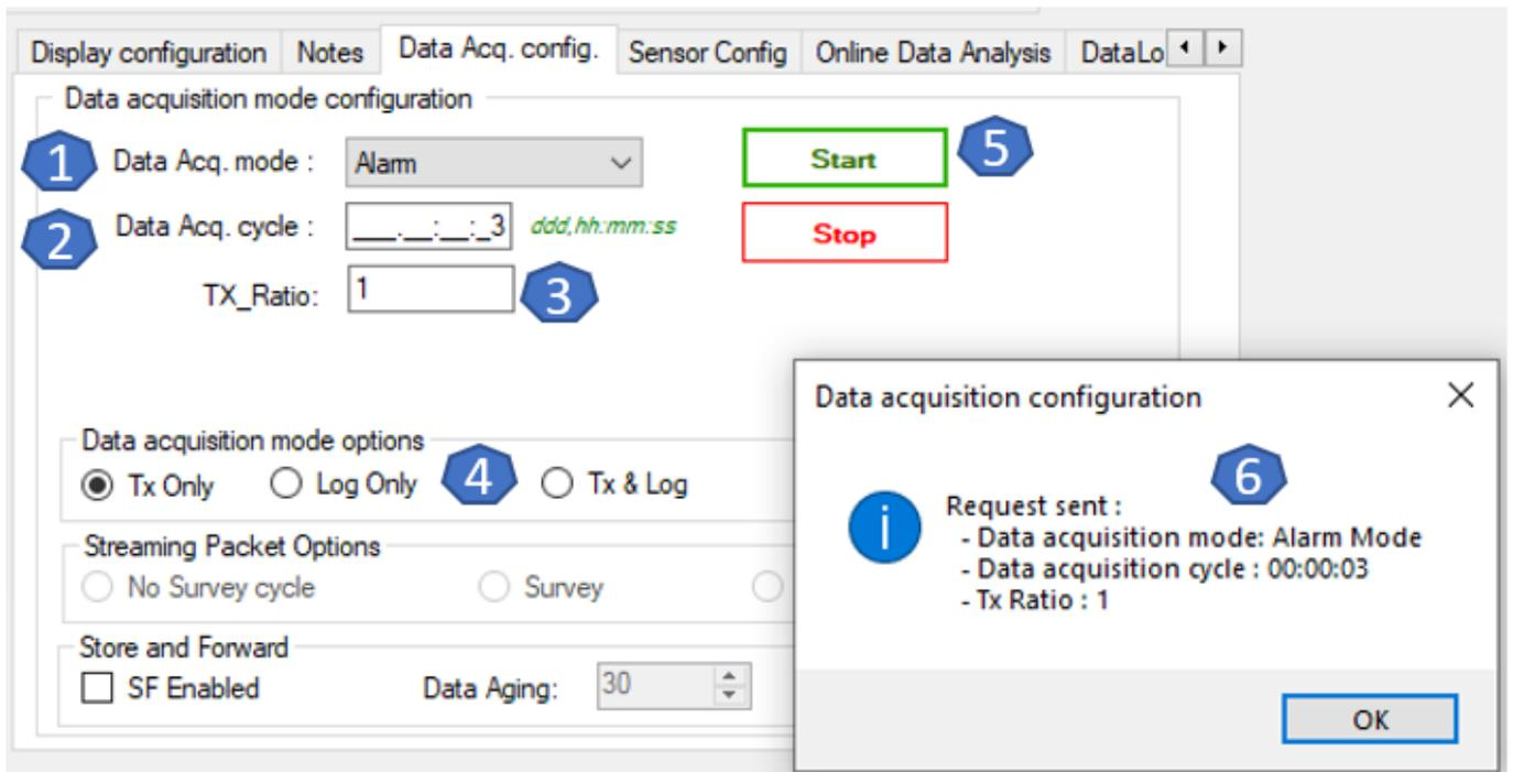
*Figure 31: alarm mode configuration*
