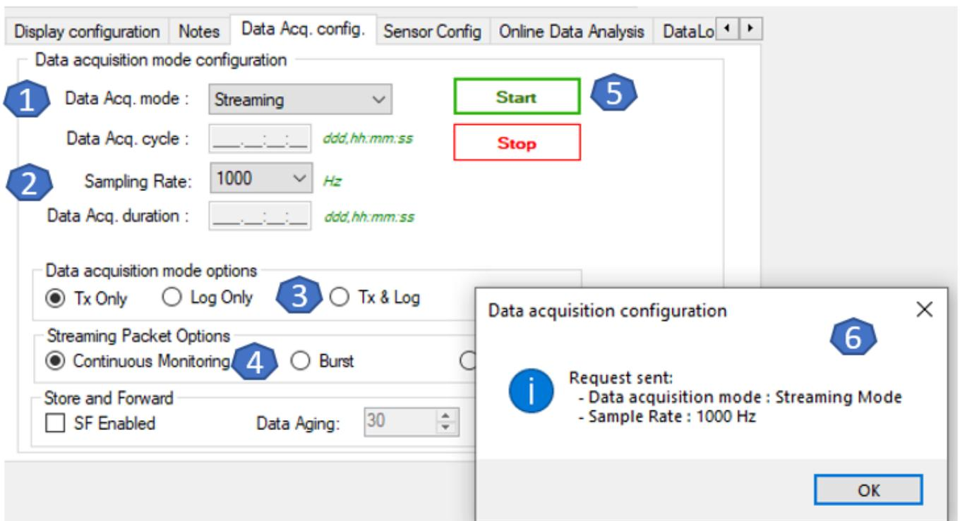
*Figure 33: Streaming mode configuration*
