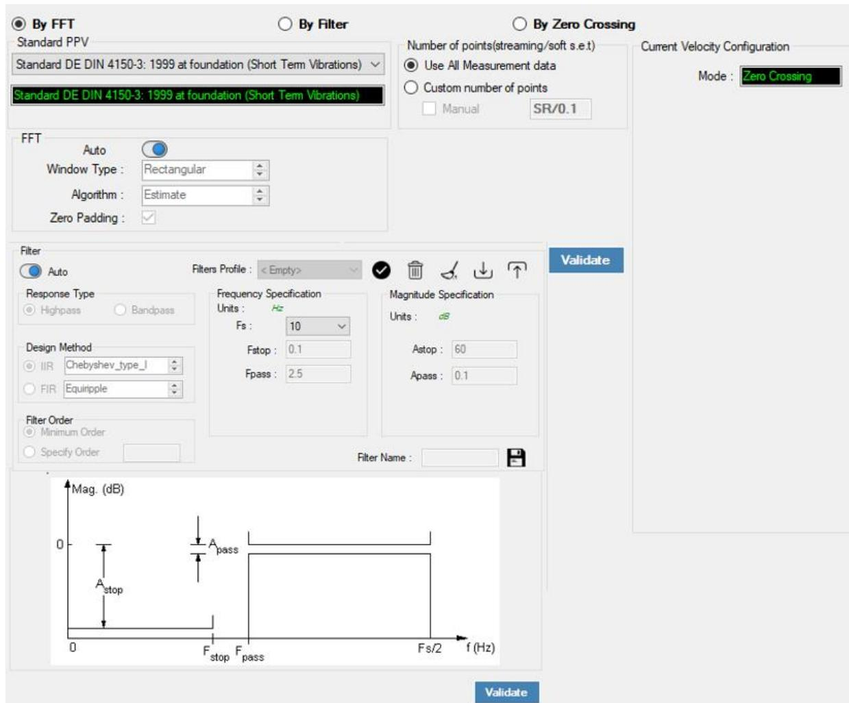
**Figure 60: Velocity Advanced Configuration**
