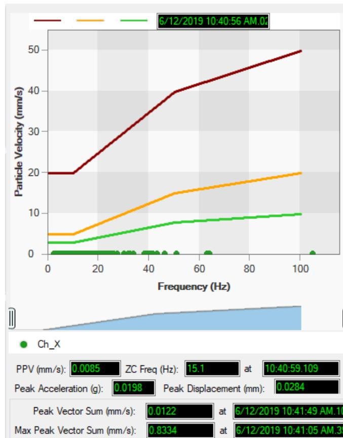
Figure 76: DIN 4150 Real Time Graph, PPV & PVS
