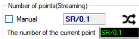
By default, the Number of Points is configured to be set automatically as Sampling Rate / 0.1 (SR/0.1).
