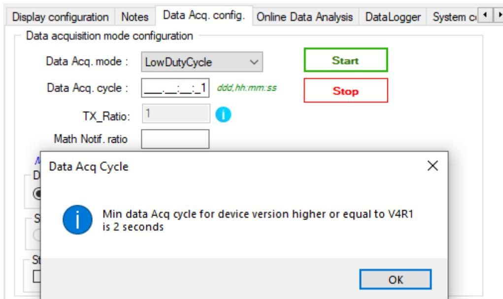
Figure 28: Minimum DAQ cycle on LDC
