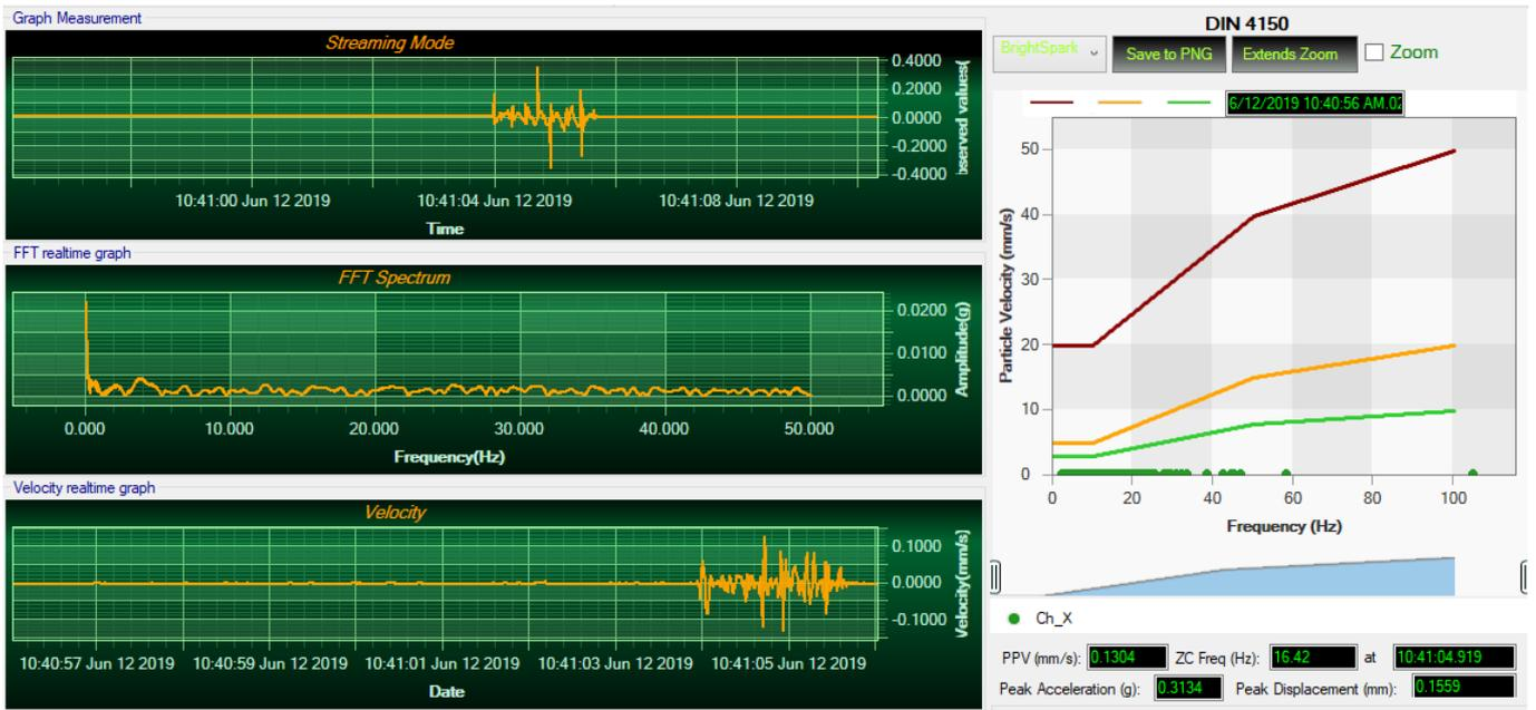
Figure 75: Velocity and FFT Graph, PPV and PVS
