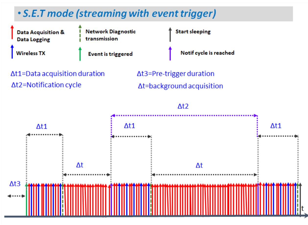
Figure 5 : Streaming with Event Trigger
