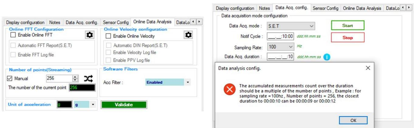
***Figure 82: DAQ duration with manual buffer seize settings***
