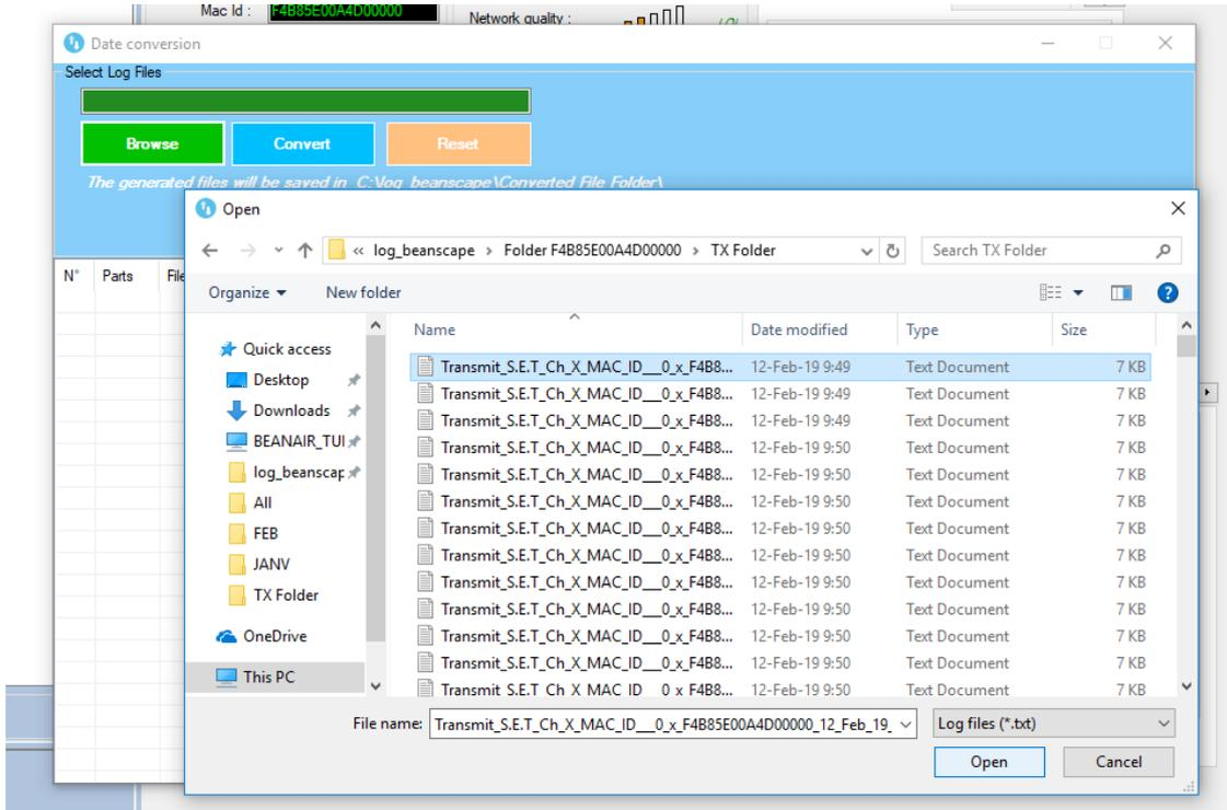
**Figure 92: Importing files into data conversion window**
