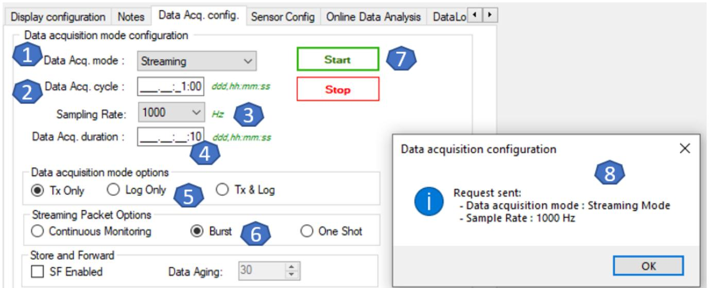
**Figure 35: streaming mode with burst option configuration**
