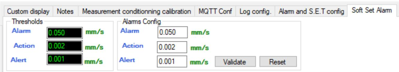
Figure 24: Soft SET alarm thresholds
