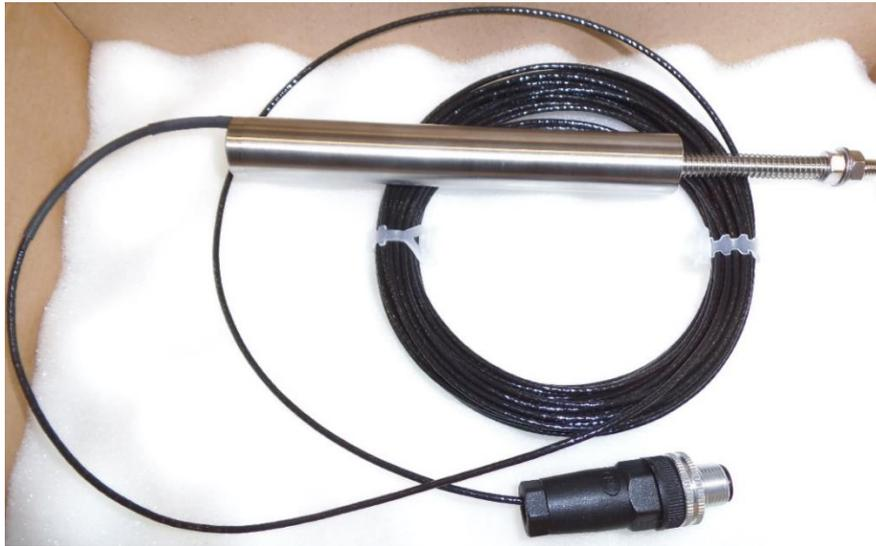
*Figure 14: LVDT sensor integrated with M12-4Pins Plug*
