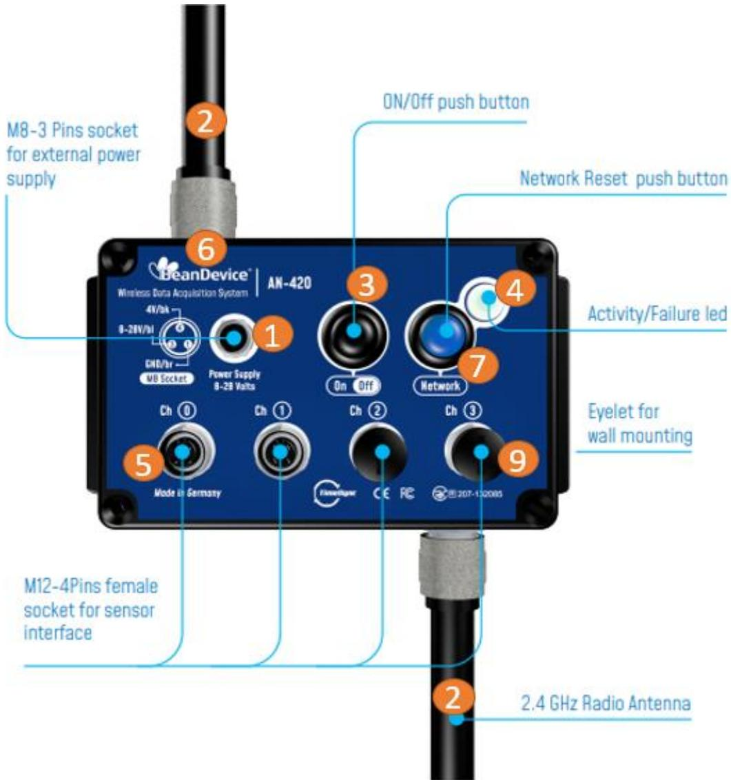
**Figure 1: Focus on BeanDevice® AN-V/AN-mV/AN-420**
