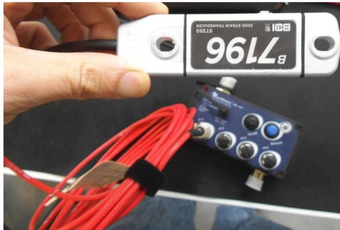
**Figure 18: Load strain transducer combines with the BeanDevice AN-mV**
