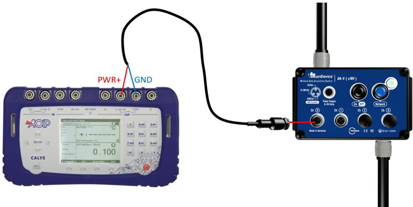
Connect the channel of the BeanDevice to the calibrator's Output: Sens+ to the V and Sens- to COM
