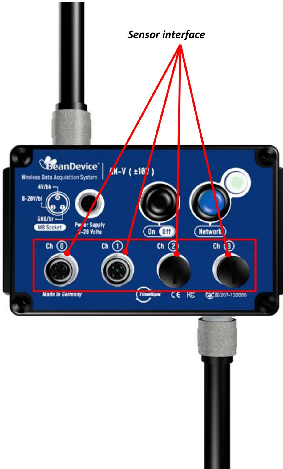
*Figure 5: M12 socket location the BeanDevice®*
