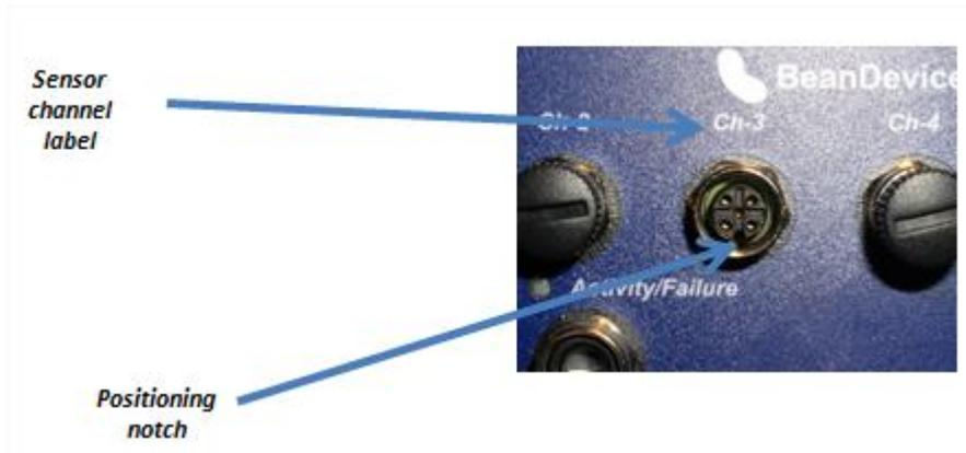
**Figure 6: M12 Socket - positioning notch**
