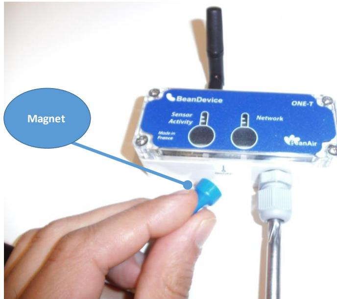
**Figure 23: Using Magnet to Power ON/OFF**
