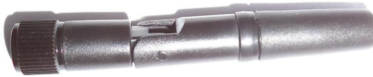
**Figure 21 : Omnidirectional 2.2dBi Antenna**
