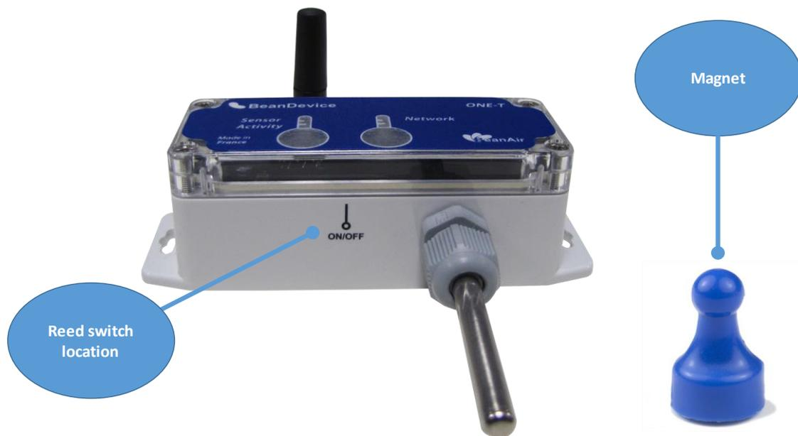
***Figure 22: Powering ON/OFF the BeanDevice®***
