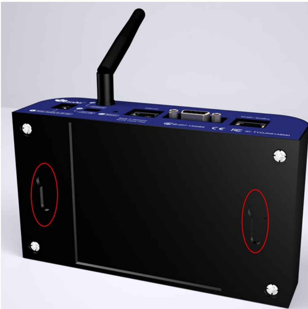
Figure 14: Slots for wall mounting
