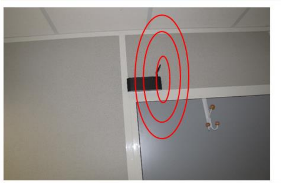
Figure 11: A BeanGateway® indoor mounted on a wall
