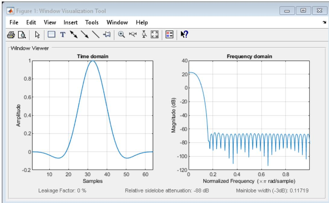
**Figure 202: Flat Top Window Graph on MatLab**
