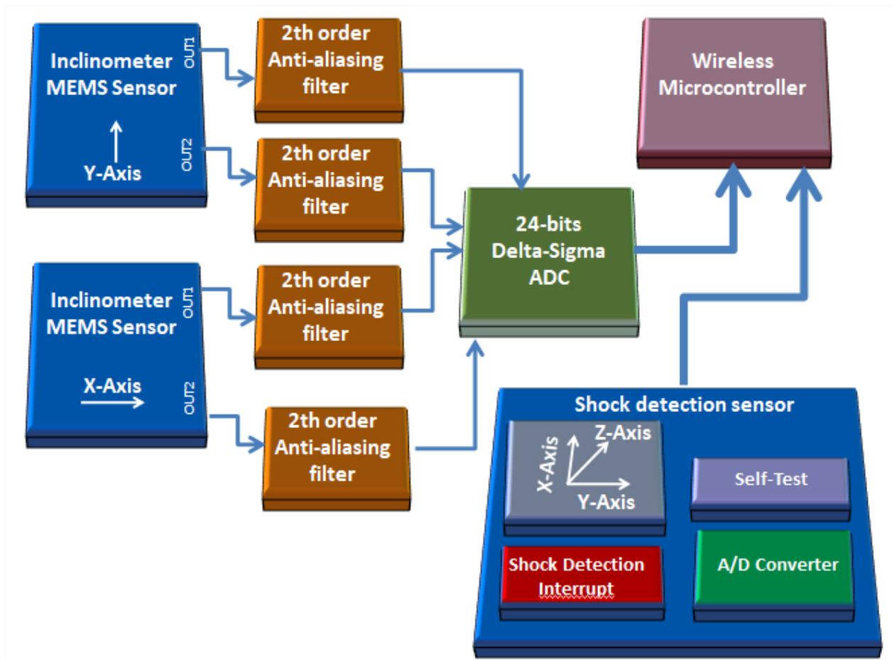
Figure 12: X-INC sensor architecture
