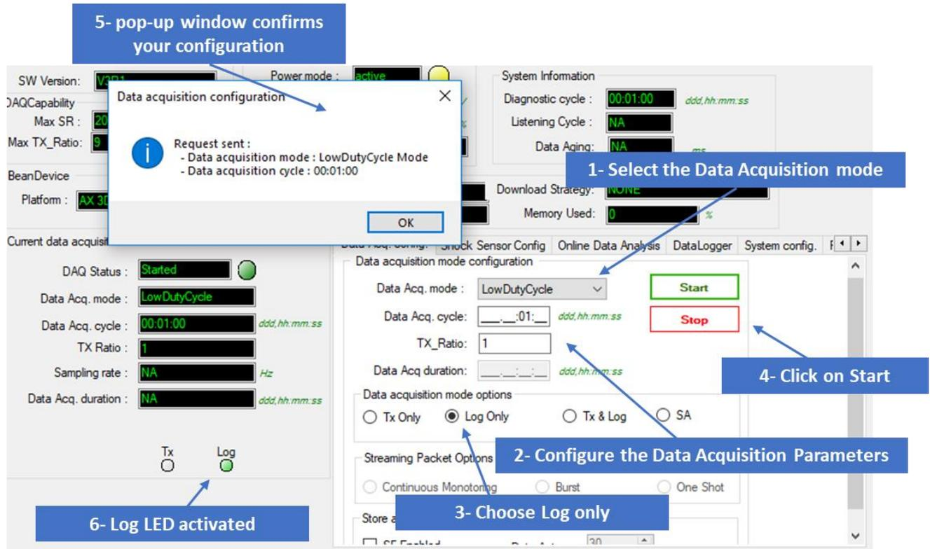
Figure 106: Overview: Data acquisition configuration scenario
