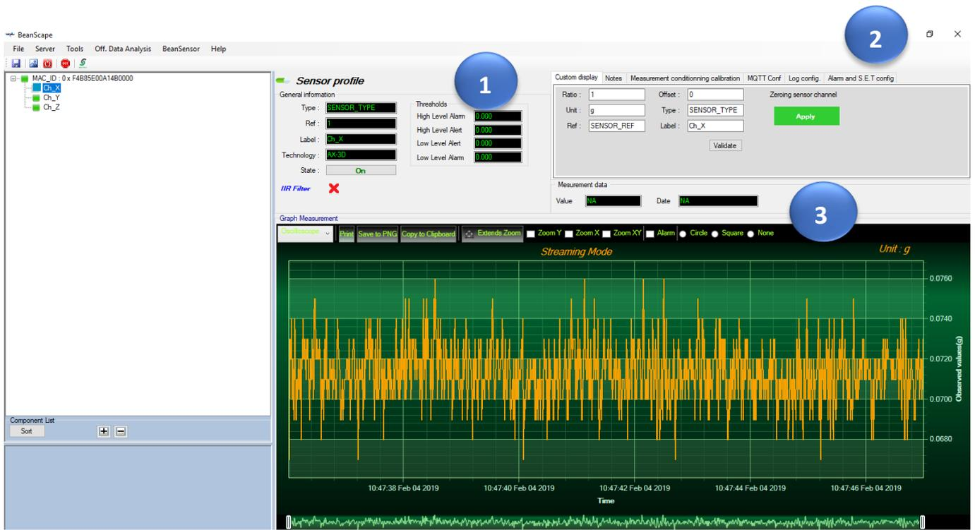
Figure 89: Overview: Sensor channel profile
