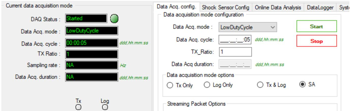
**Figure 109: BeanDevice Configured with LDCDA mode with Stand Alone**
