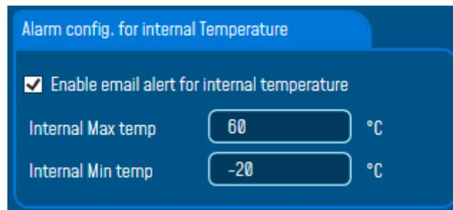
*Figure 169: system alarm settings*
