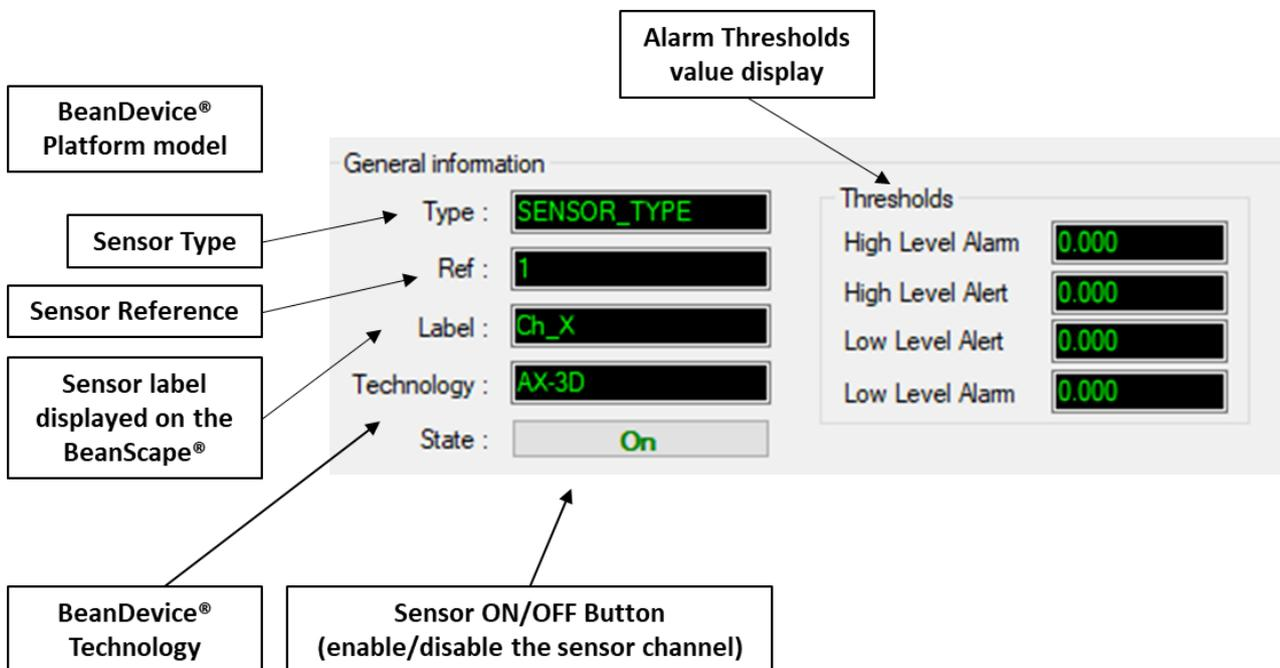
Figure 90: Sensor channel General information frame
