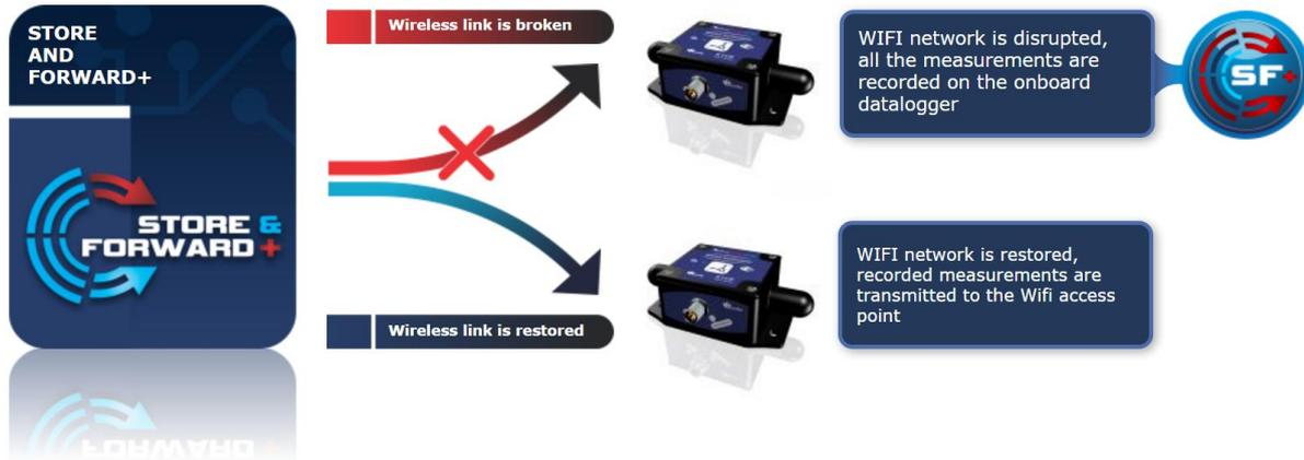
**Figure 13 : Store and Forward+ mechanism**
