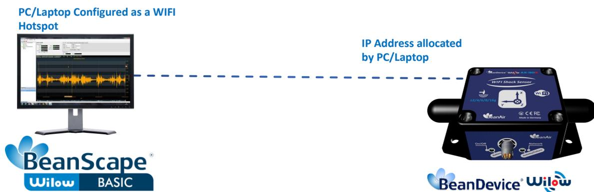
*Figure 25: Direct connection to a PC/Laptop*
