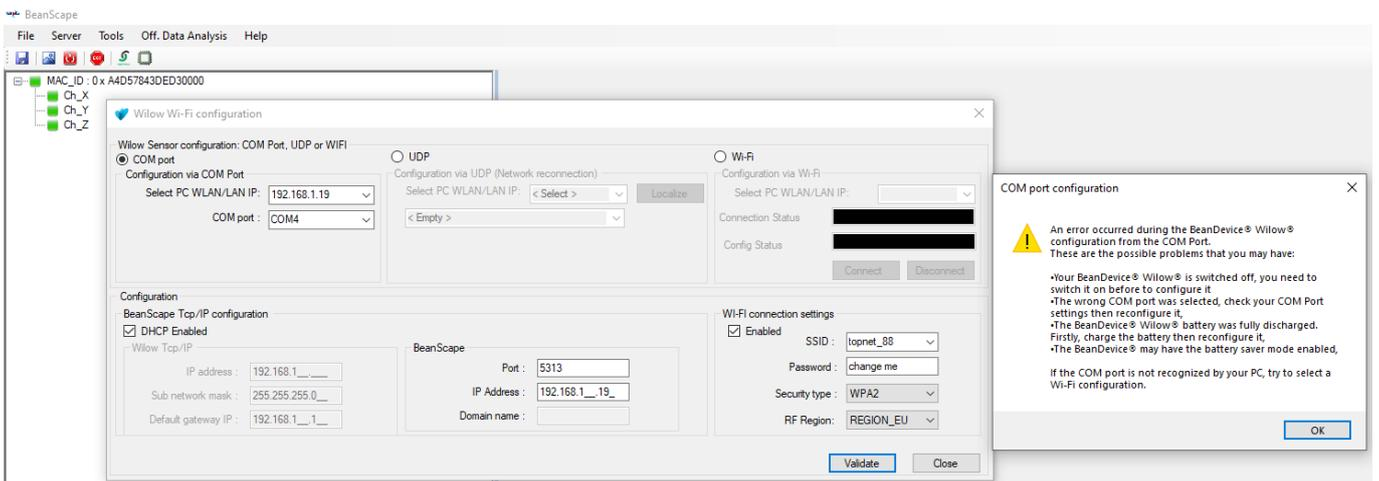
**Figure 35: BeanScope® WiLow configuration error**
