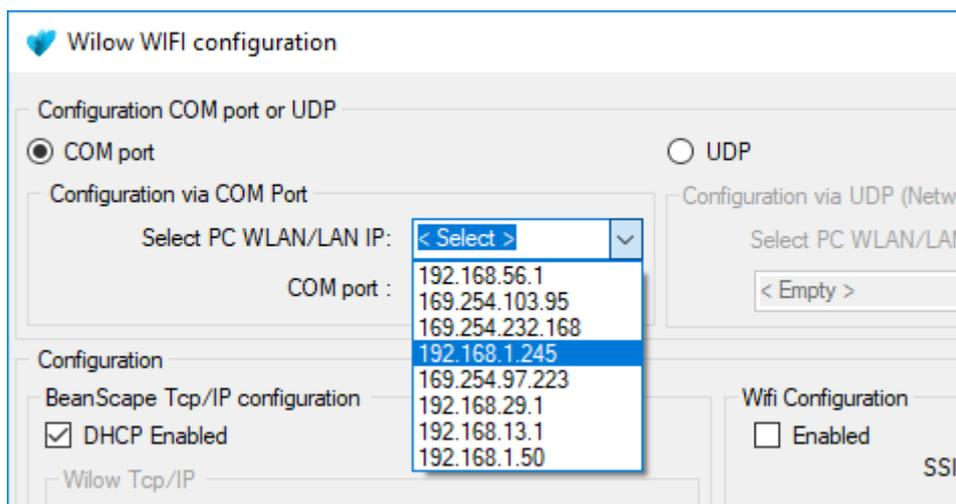
**Figure 29: COM/LAN Port setting**
