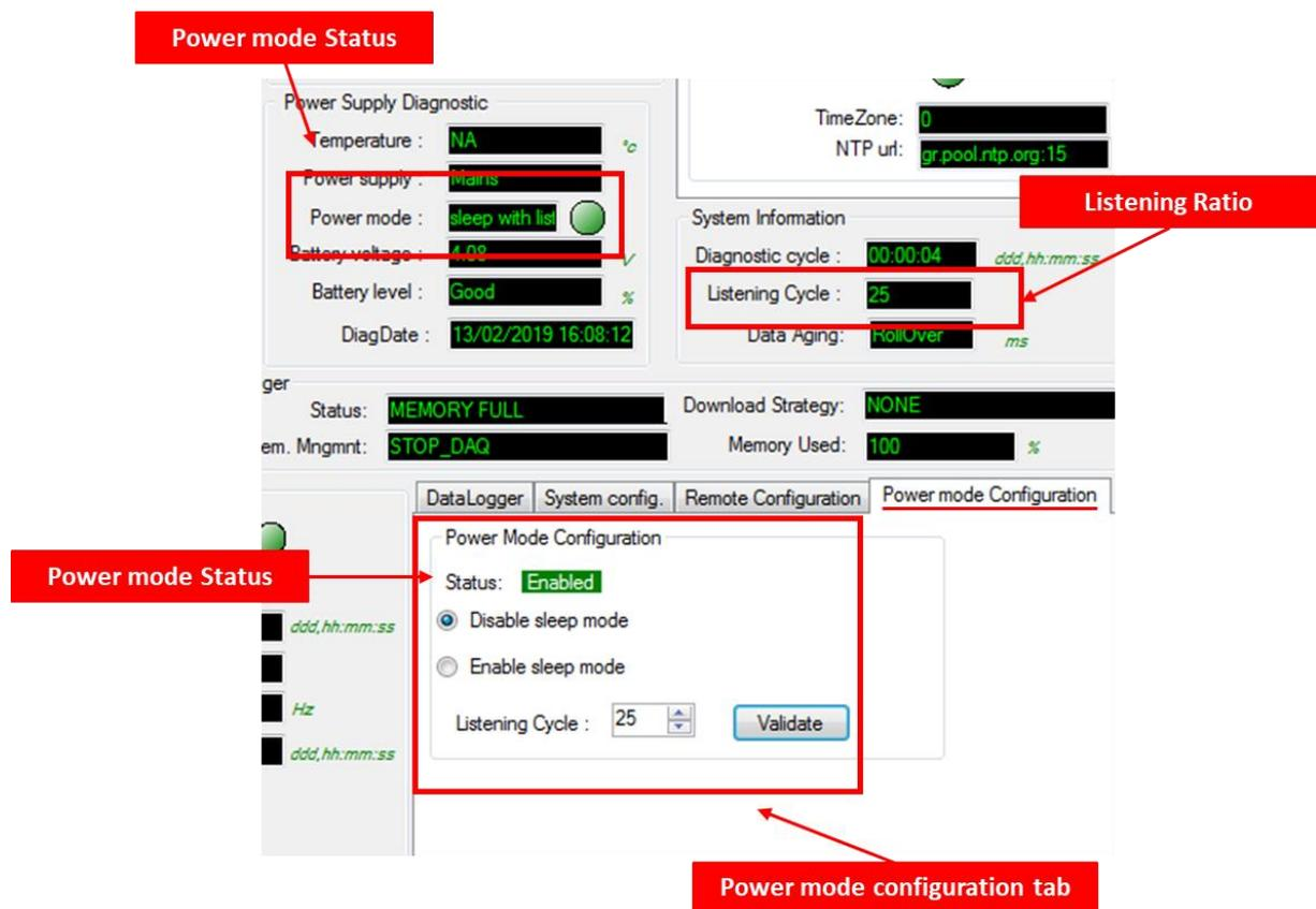
**Figure 76: Power mode management (display features)**
