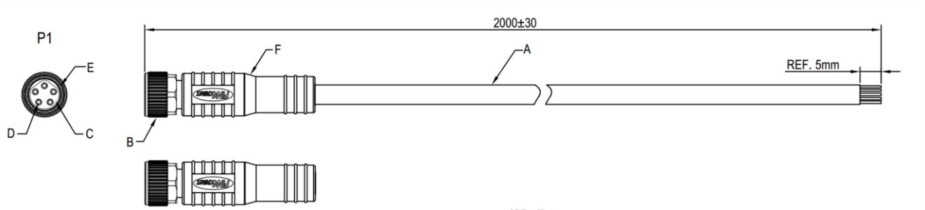
***Figure 22: M8-5Pin/M8-6Pin cable***
