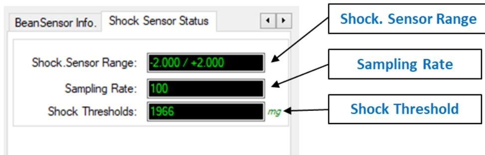
**Figure 62: Shock Sensor status frame**
