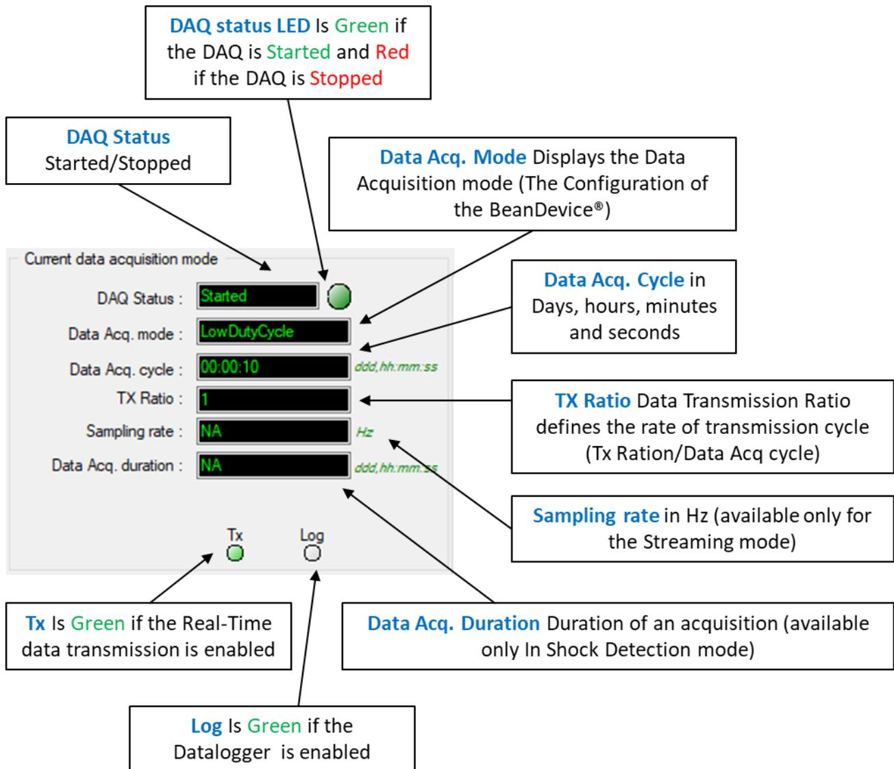
**Figure 65: Frame curent data acquisition mode**
