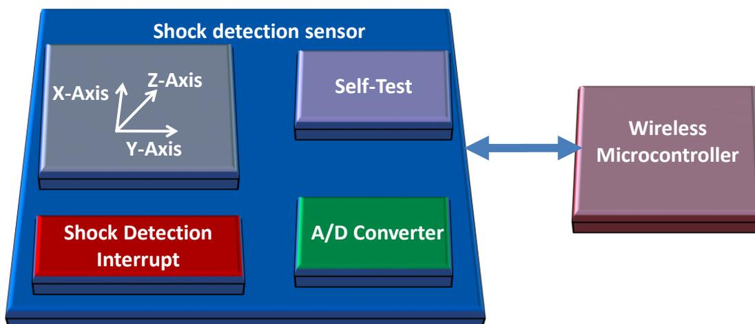
**Figure 9: BeanDevice® WiLow® AX-3DS - MEMS Sensor Architecture**
