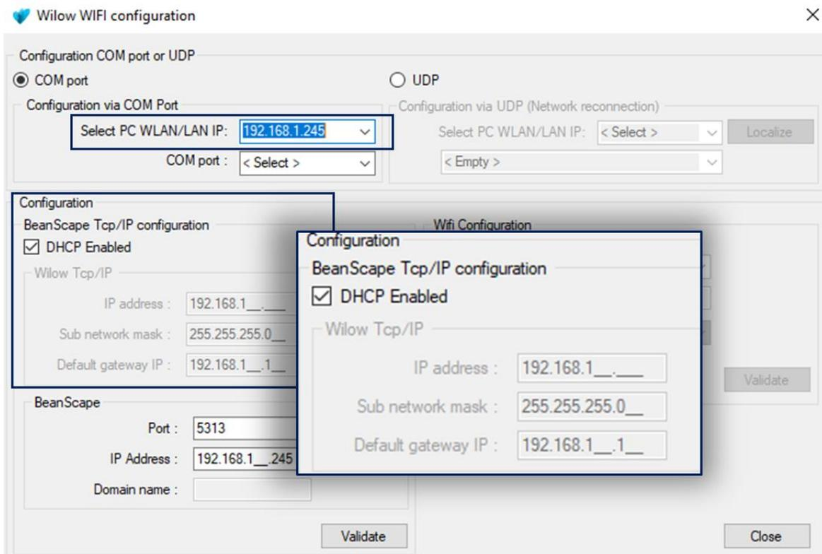
**Figure 30: BeanDevice® WiLow IP setting**
