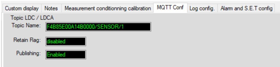
**Figure 96: Sensor MQTT configuration tab**
