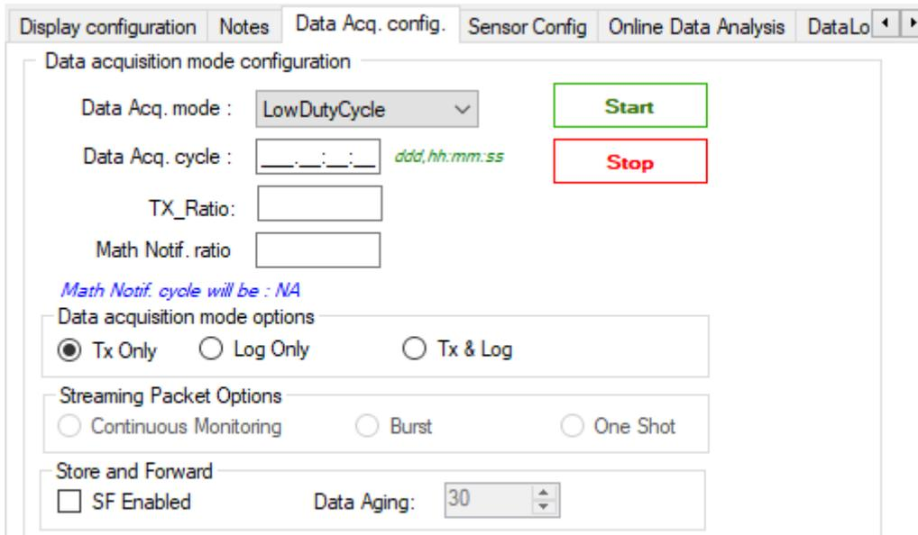
**Figure 69: Data Acquisition configuration tab**
