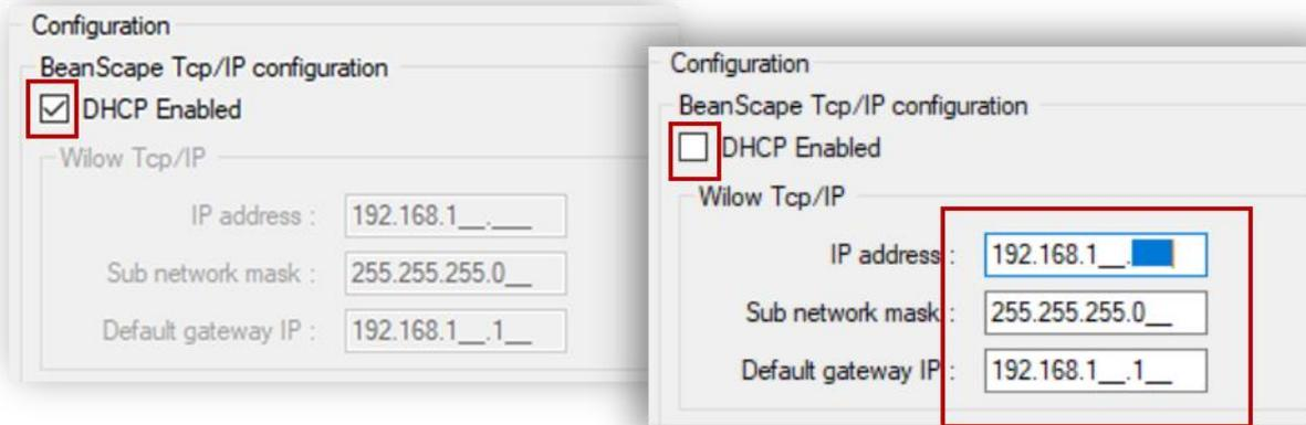
**Figure 32: BeanDevice® Wilow® DHCP/Static IP**
