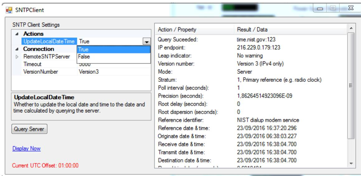
**Figure 158: SNTP Client configuration**
