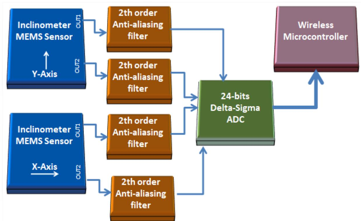
**Figure 6: BeanDevice® WILO® HI-INC - MEMS Sensor Architecture**
