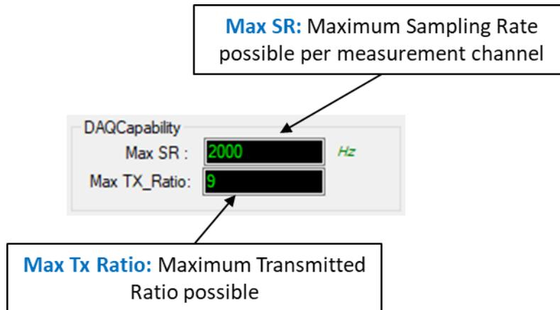
**Figure 57: DAQ Capability frame**
