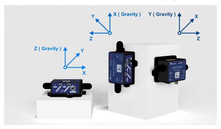
The Axis with the Gravity is not taken into account in the Automatic Range
