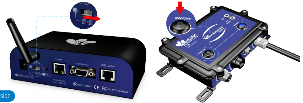
Figure 10 : Turn on the BeanGateway®
