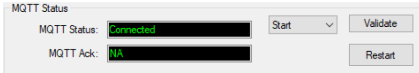
Figure 29: Start the MQTT server
