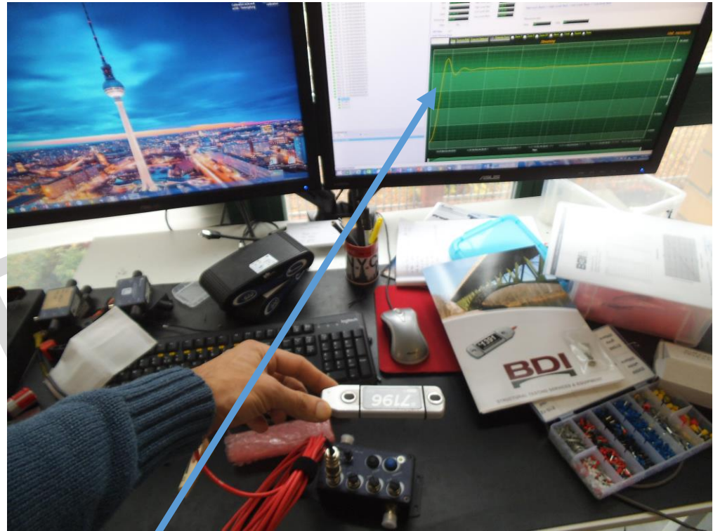
Load strain sensor reacting to a traction effort
