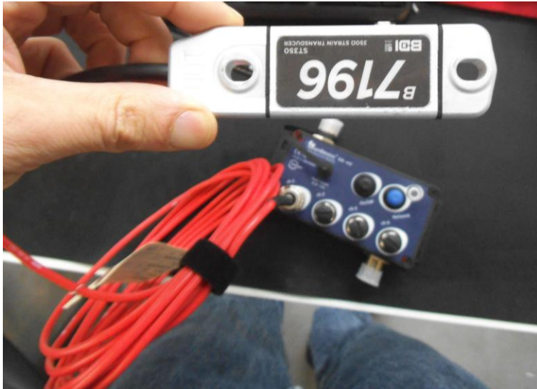
Load strain transducer combines with the Beandevise AN-mV
